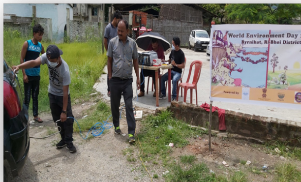
Emission test of Petrol driven vehicle in progress
