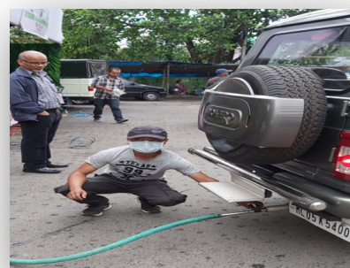
Emission test of Diesel vehicle in progress
